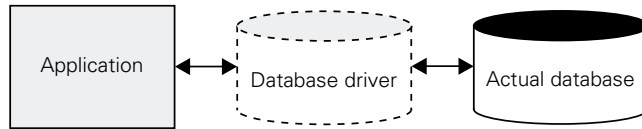
Figure 14.1 The application talks to the driver, and the driver talks to the database.
