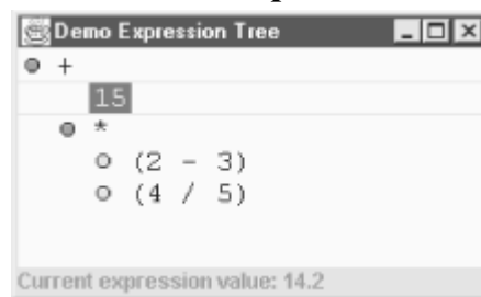
Figure 17.8. A tree event listener label that updates the current value of our expression
