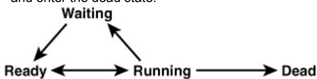
Figure 8.2: Interaction between thread states.
