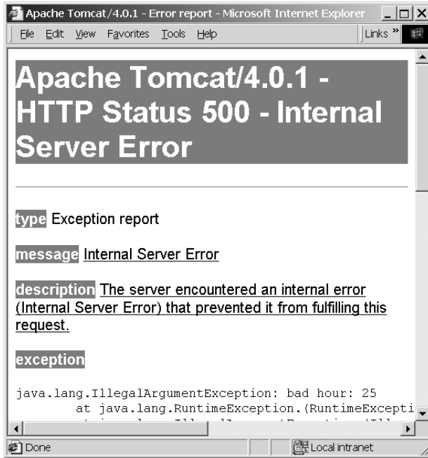
Figure 15.2 Page authors can see the error messages that tag developers write. In this case, the text “bad hour: 25” comes from the TimeTag handler, a custom tag handler we wrote earlier in this chapter. Tag authors should take this opportunity to provide helpful, informative error messages when appropriate.
