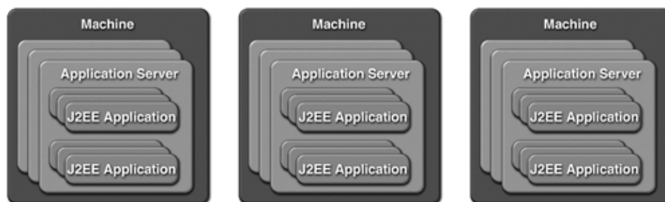
Figure 8.3. Deploying HP Bluestone Total-e-Server on Multiple Machines
