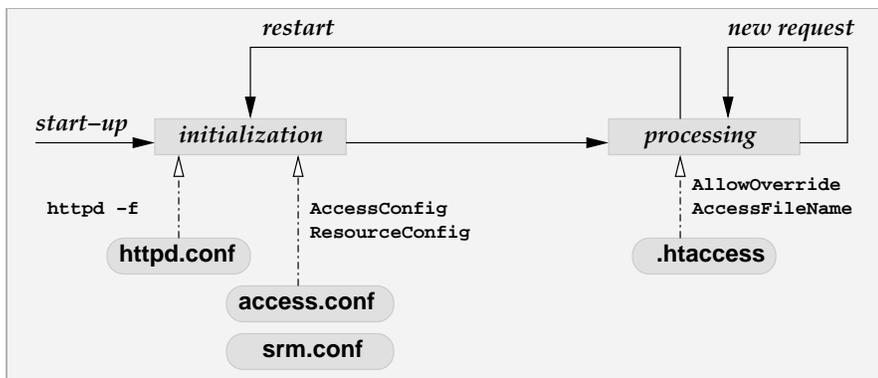
Figure 4.2: Processing of configuration files
