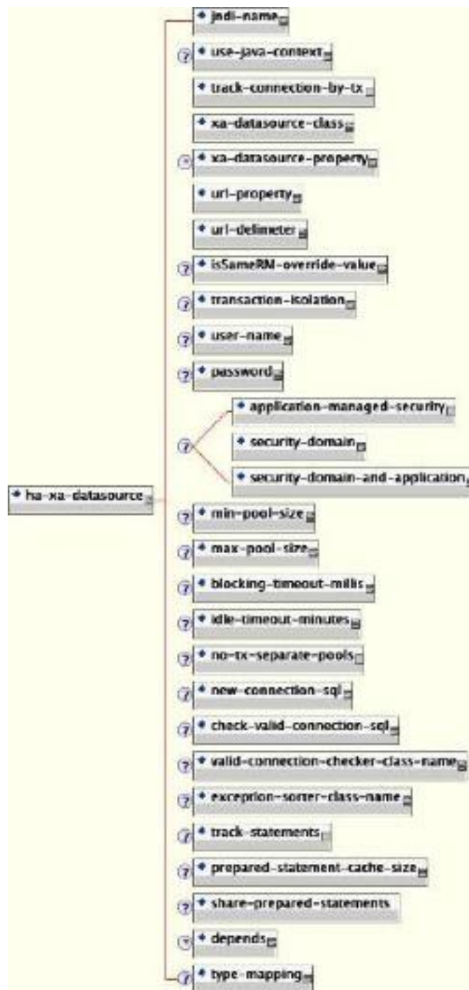
Figure 5.10. The schema for the experimental XA Datasource with failover
