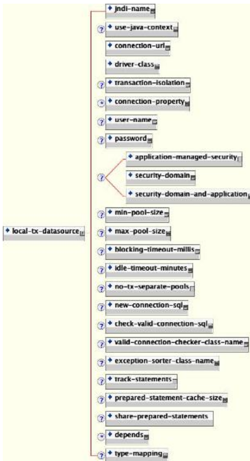
Figure 5.7. The non-XA DataSource configuration schema
