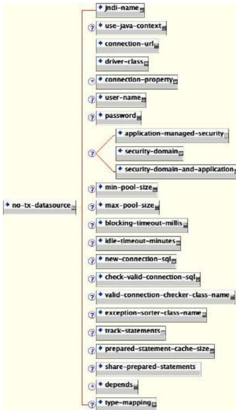
Figure 5.6. The non-transactional DataSource configuration schema
