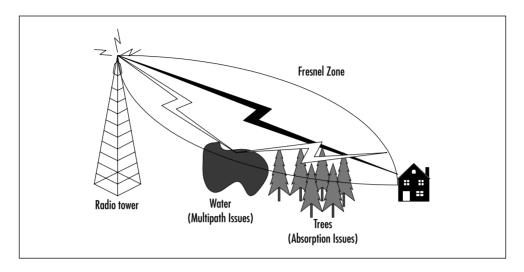
Figure 4.2 Fresnel Zone: Absorption and Multipath Issues
