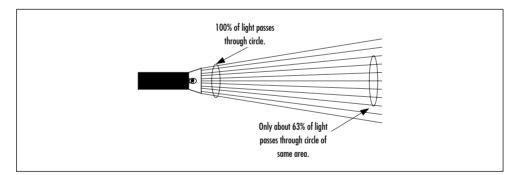
Assuming the omnidirectional light fixture in Figure 2.8 and the flashlight in Figure 2.9 both transmitted the same amount of energy, it is easy to see that the flashlight gets a stronger signal to a receiver that is the same distance away. We will talk about directional antennas in more depth later in this chapter.
