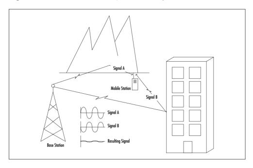
Figure 2.12 Illustration of Multipath Scattering
