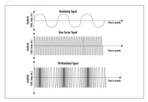
Figure 2.3 Frequency Modulation (FM)
