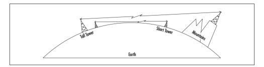
Figure 2.10 How Towers Can Extend Transmission Distance
