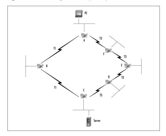
Figure 3.7 Static Routing in a Multihop, Multipath Network
