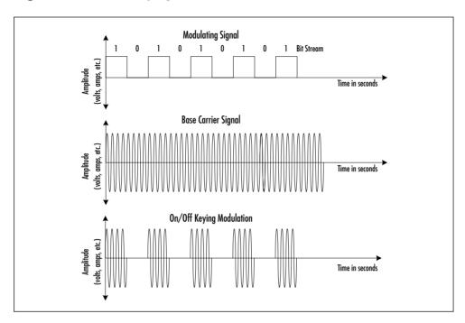
Figure 2.4 On/Off Keying (OOK) Modulation
