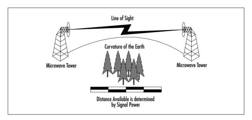
Figure 4.5 Point-to-Point Microwave
