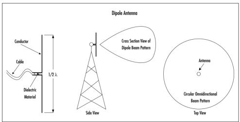
When the antenna is not near half the wavelength, the performance of the antenna is drastically affected due to a mismatch in characteristic impedances and standing wave ratios.
