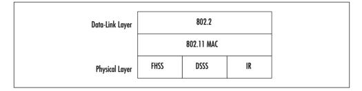
The three physical layer options for 802.11 are infrared (IR) baseband PHY and two radio frequency (RF) PHYs. Due to line-of-sight limitations, very little development has occurred with the Infrared PHY. The RF physical layer is composed of Frequency Hopping Spread Spectrum (FHSS) and Direct Sequence Spread Spectrum (DSSS) in the 2.4 GHz band. All three physical layers operate at either 1 or 2 Mbps. The majority of 802.11 implementations utilize the DSSS method.
