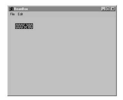
Figure 12.6. The BeanBox main container with a modified LED display bean.
