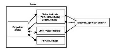
Figure 4.3. The role accessor methods play in allowing external access to a bean's properties.
