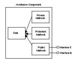
Figure 2.2. The relationship between interfaces and methods in a JavaBeans component.
