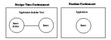
Figure 8.1. The difference between shipping a bean for use in runtime and design-time environments.
