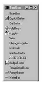
Figure 11.2. The BeanBox ToolBox window with the meter bar bean added.
