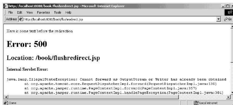
Figure 6.2 The results of accessing flushredirect.jsp
