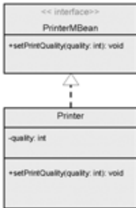
Figure 4.1 The simplest case: direct implementation of an MBean interface. The resulting management interface is the methods contained in the PrinterMBean interface.
