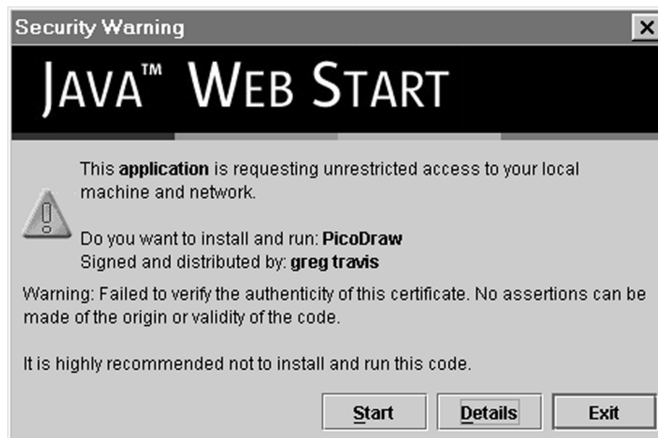
Figure 4.2 The JAWS environment asks the user's permission before the signed application is allowed to execute.
