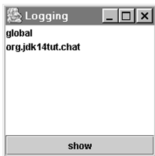
Figure 5.5 The main window of LoggerGUI. This window shows a list of the loggers currently instantiated within the logging system. Selecting one of them and clicking show brings up a logging window for that logger.
