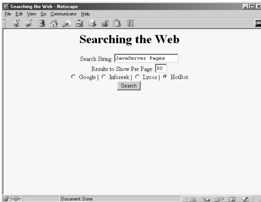
Figure 8-4 Result of SearchEnginesFrontEnd servlet. Whatever options you specify will be the initial choices next time you visit the same servlet.
