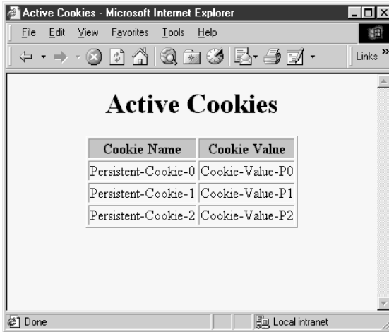
Figure 8-3 Result of visiting the ShowCookies servlet within an hour of visiting SetCookies in a different browser session.
