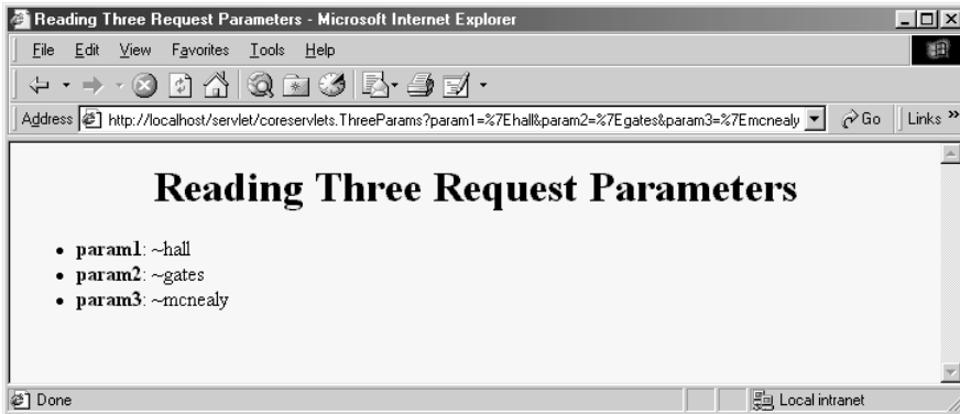
Figure 3-2 Output of ThreeParams servlet.
