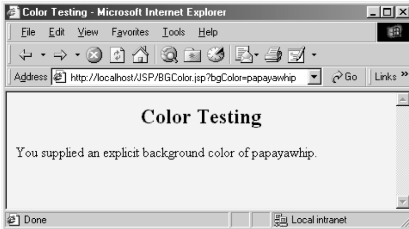
Figure 10-4 Result of BGColor.jsp when accessed with a bgColor parameter having the X11 color value papayawhip .
