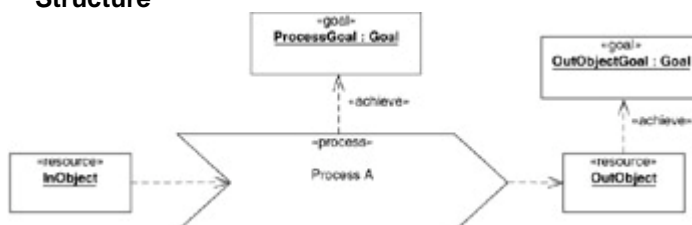
Figure 8.2: The structure shows that a goal can be allocated to a process or an object.
