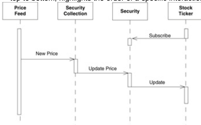
Figure 4.20: A sequence diagram showing how a price update of a security is distributed to other resources.
