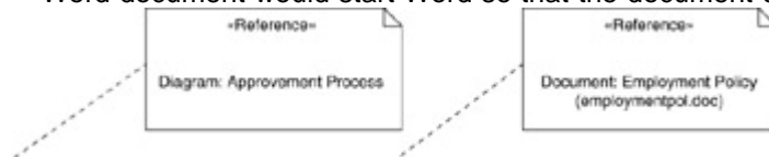
Figure 3.16: A reference note allows the modeler to visually reference another diagram or document in a standard manner.
