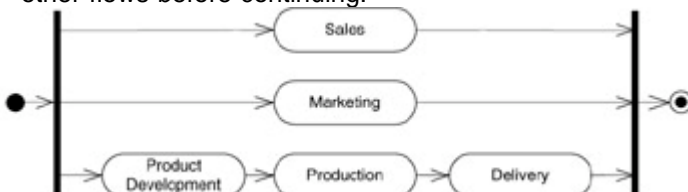
Figure 2.27: Sales and marketing are done in parallel with the activity series product development, production, and delivery. In the automotive industry this is called concurrent engineering; marketing is done in parallel with sales, product development, and so on.
