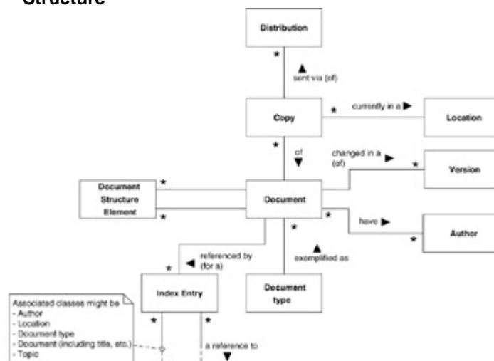
Figure 7.15: The structure for the Document pattern. It captures motivation, and includes index, document type, and document structure elements.
