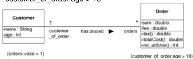
Figure 5.3: Role names in associations are used to navigate from the context to other classes.
