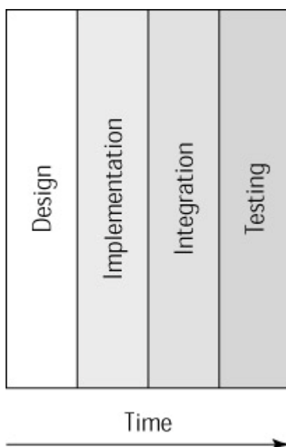
Figure 1-1: The waterfall development process moves through each phase of development until final release.
