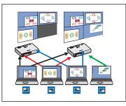
This arrangement can be used when you wish to simultaneously display multiple presentations using multiple projectors.
