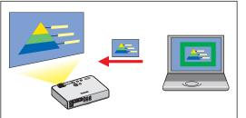
By using the selective area window, you can specify the necessary information alone from the computer screen, and display it on the projection screen.
